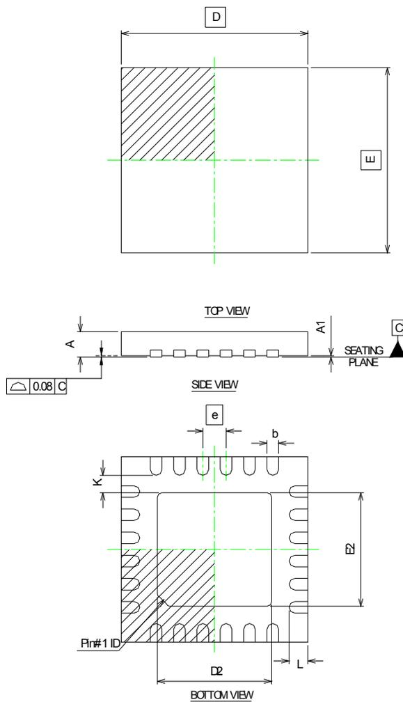
**Table 23. QFN-24 EP (4x4) package mechanical data**
