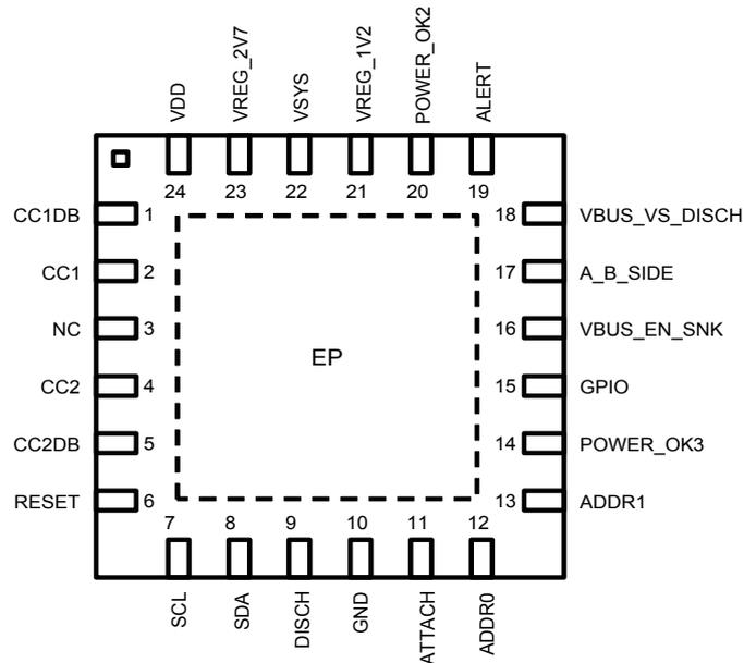
**Figure 3. WLCSP-25 pin connections (top view)**
